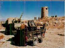
Weapons left behind by Soviet army now are used on all sides of Afghan civil war: (from left) Mujahideen fire-support unit comprises truck-mounted 23mm anti-aircraft guns and jeep-mounted 140mm multiple-rocket launcher (MRL). T-62 tank in anti-Taliban
